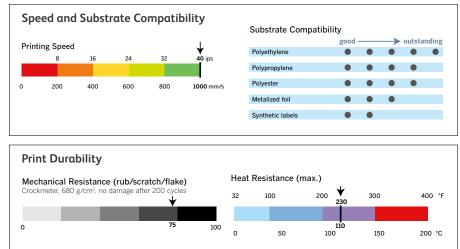
Videojet evaluation of observed performances of the Long Length Ribbon with optimized printer setting and receptors.
